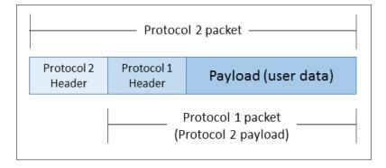
This is called **encapsulation**, and as we'll see shortly, it is a powerful mechanism for structuring network traffic.
