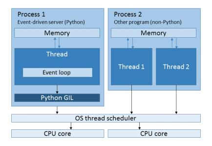
Although the GIL and the OS thread scheduler are shown here for completeness, in the case of an event-driven server, they have no impact on performance because the server only uses a single thread. The scheduling of I/O handling is done by the application.
