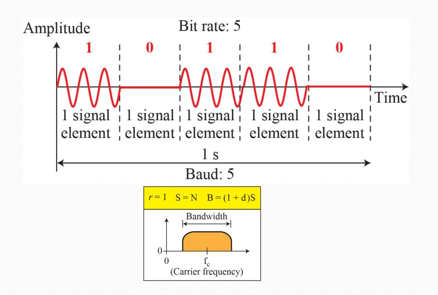
The ASK technique is used to transmit digital data over optical fiber, where one signal element is represented by a light pulse while the other signal element is represented by the absence of light.
