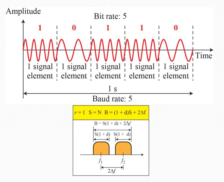
The most common form of **FSK** is binary FSK (BFSK), in which the two binary values are represented by two different frequencies near the carrier frequency, as shown in the Figure.
