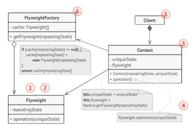
The Client calculates or stores the extrinsic state of flyweights. From the client's perspective, a flyweight is a template object which can be configured at runtime by passing some contextual data into parameters of its methods.
