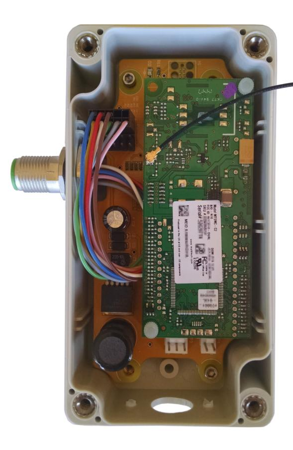
In the preceding diagram, the lower circuit board implements the functionality of the device (monitoring cryogenic liquids, in this case). On this board, the power supply system, sensor electronics, and a low-cost, 16-bit microcontroller are found. A cellular modem is located on the top circuit board, which plugs into a socket on the lower board.
