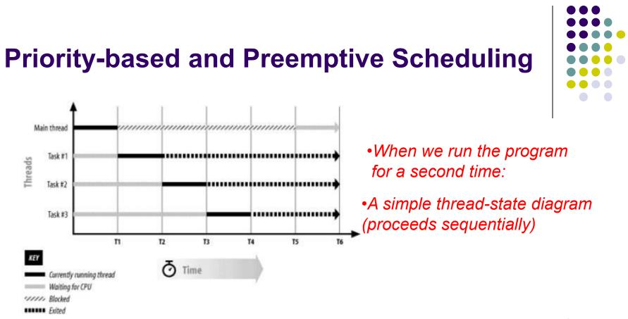
The main thread is the currently running thread until it blocks at time T1. At that point, one of the task threads becomes the currently running thread; it remains the currently running thread until time T2 when it finishes and transitions to the exiting state. Another task thread becomes the currently running thread, and the cycle continues until all threads have completed.
