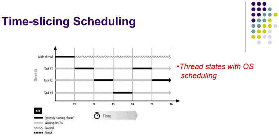
The thread scheduler on that OS, in addition to being priority-based and preemptive, is also time-slicing.
