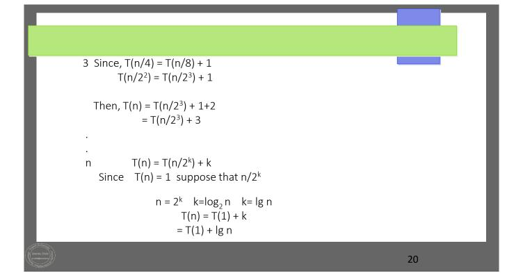
The closed end formula  $= 1 + \lg n$ The running time T(n) is O(lg n).
