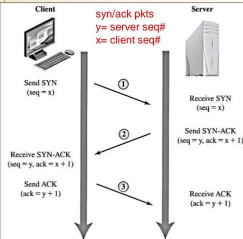
Figure 7.2 TCP Three-Way Connection Handshake
