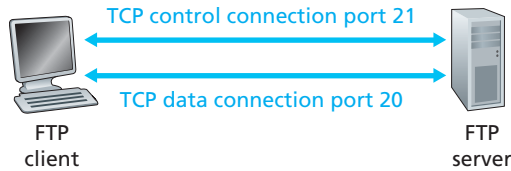
Figure 2.15 ♦ Control and data connections
