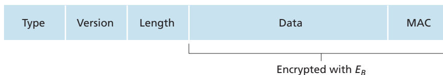
Figure 8.26 ♦ Record format for SSL
