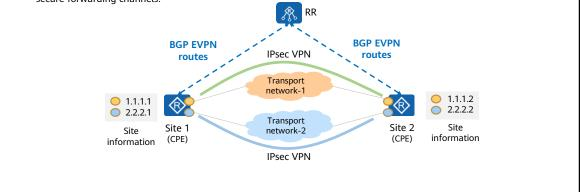
• Overlay VPN routes include site VPN route prefixes, next-hop route information, and IPsec key pairs required for data encryption of data channels between CPEs.
