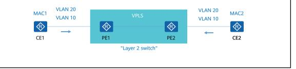
VPLS does not support all-active access or load balancing and implements slow fault convergence. For details, see materials of the HCIE-HCIE-Datacom Ethernet VPN and RFC 7209 titled "Requirements for Ethernet VPN (EVPN)."
