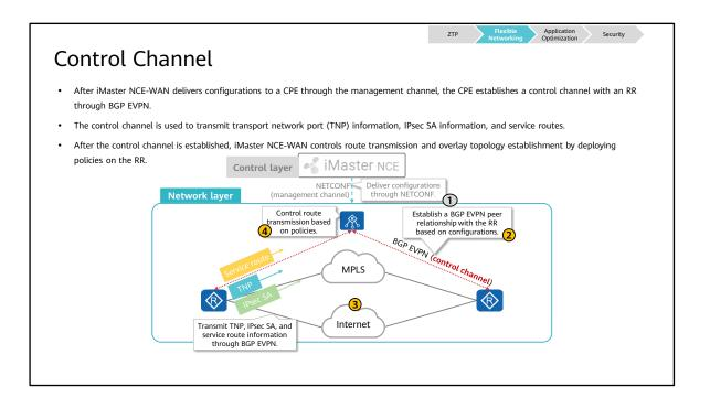
• A TNP is a WAN port on a CPE used for connecting to a transport network. The key TNP information includes the site ID, CPE router ID, transport network ID, public IP address, private IP address, and tunnel encapsulation mode.
