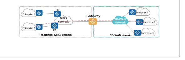
A gateway's role name varies depending on the service scenario. For example, a gateway connecting SD-WAN sites to legacy sites is an interworking gateway (IWG), as shown in the above figure. A gateway connecting SD-WAN sites to a cloud is called a cloud gateway. In addition, functions of a gateway can be extended. A gateway that connects Point of Presence (POP) sites for building a POP network is referred to as a POP gateway.
