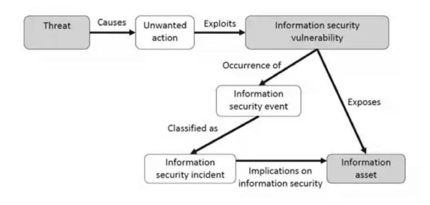
Figure \_ 1. Relationship of objects in an information security incident (ISO/IEC 27035:2011)
